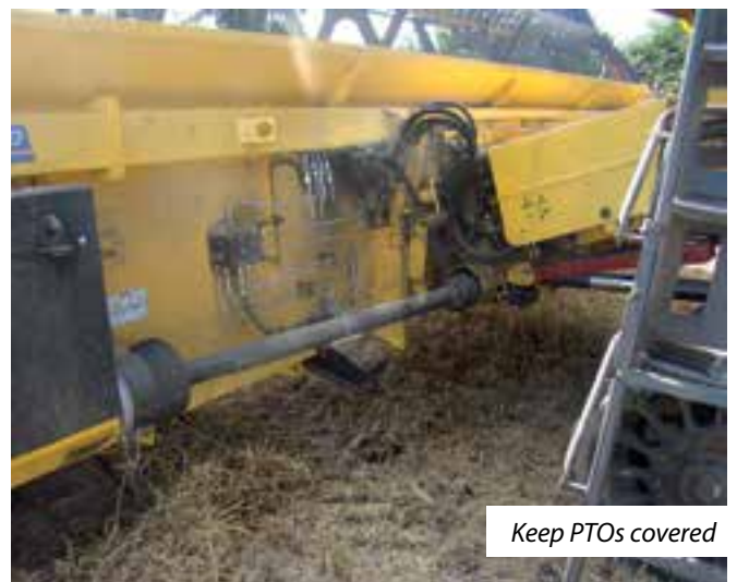
Switch off for maintenance
